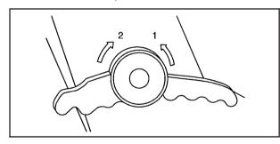
Release the rear set of seat hooks from the floor pins by pulling up on the rear part of the lever (indicated as 2 on the handle side cover). This enables the seat to be tumbled forward.
